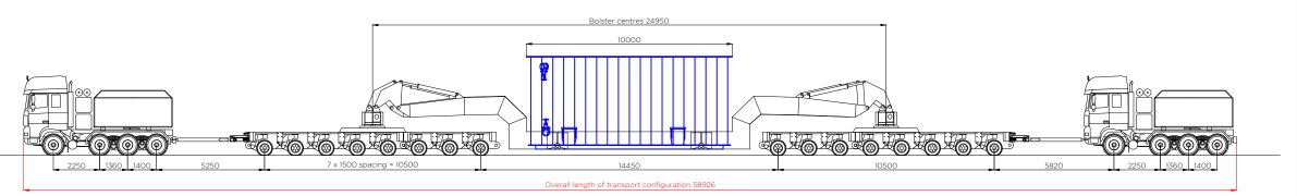
Elevation view - 16 axle girder frame trailer - concept model only Indicative 150 te transformer Scale 1:200
